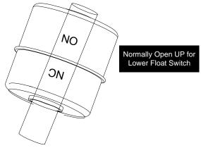
To replace the lower float switch, remove the split ring and flip the float to the Normally Open position. The wiring harness must be re-terminalized with the provided push-on terminals.
